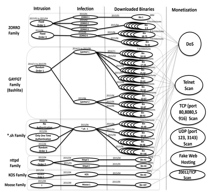
Figure 29 - Overview of Observed Attacks by IoTPOT and IOTBOX
